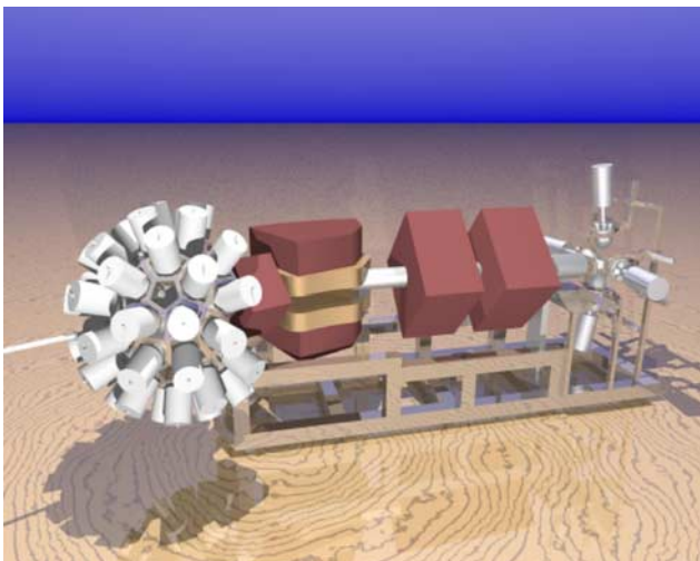
Fig. 7. An impression of the JUROGAM array of 45 EUROGAM Phase-I Ge detectors situated at the target position of RITU.
